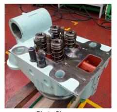
Photo Shown: After pusher is inserted into cylinder head
